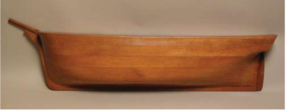
9. LAMINATED NANTUCKET WHALER HALF HULL OF THE “NAVIGATOR”, built in 1841 in Medford, Mass. For Mathew Crosby, model made by Charles F. Sayle, 1963. 46 in. x 10 in.
